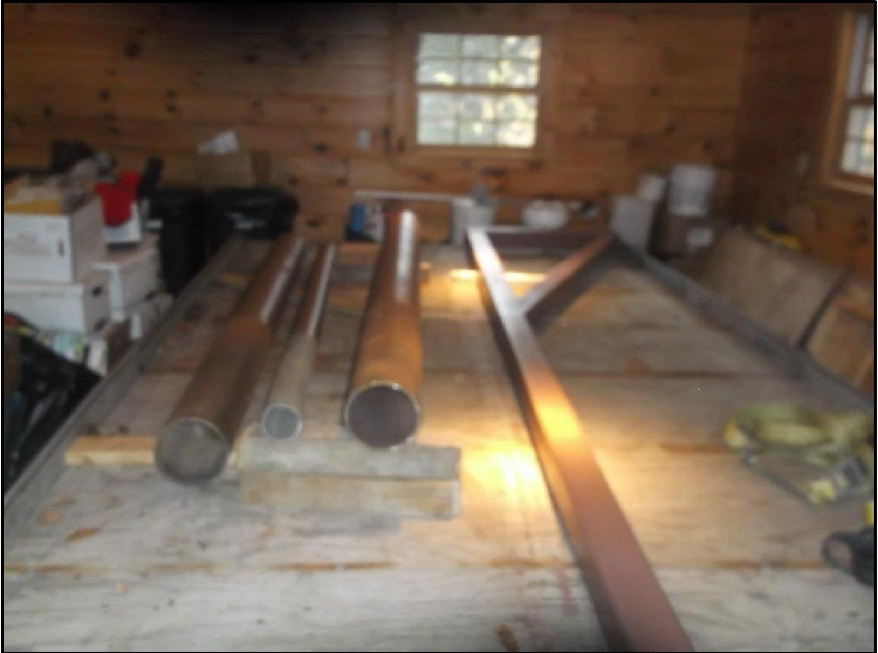
**Gate sanded and primed ready for installation. Steel plates will be welded on the bottom of the posts just prior to installation so they cannot tilt. The bottom 3-feet of the posts were not prepped or painted since they will be underground.**
