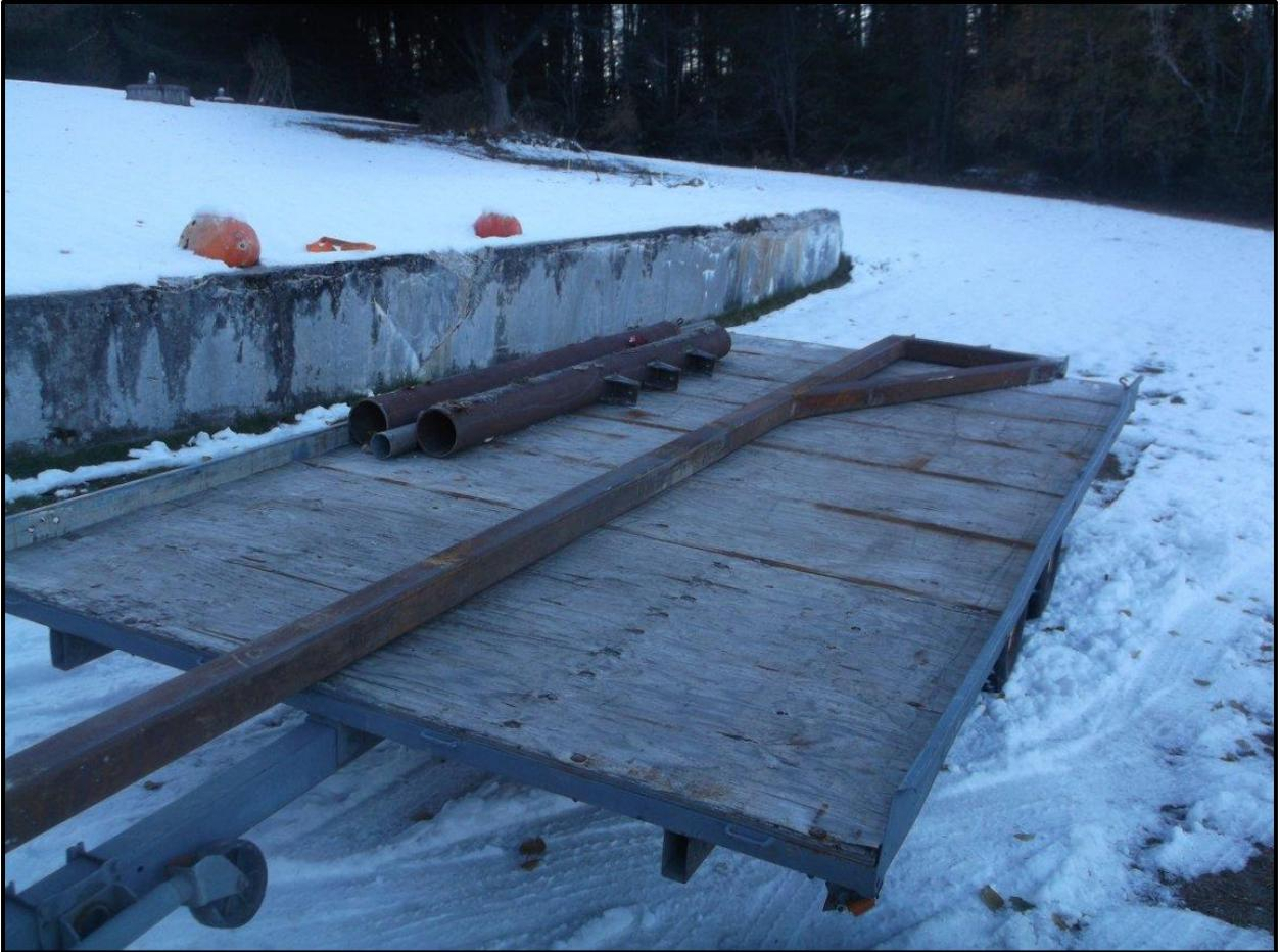
**New steel gate loaded on trailer ready for transport. Even though scrap steel was used, it will be just like new after a thorough sanding and a coat of oil-based primer.**
